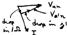
Clearly  $|V_{a'n}| < |V_{an}|$
