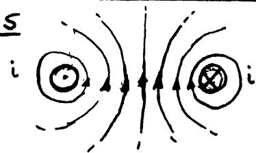
The flux linkages due to the current in the left conductor is  $\approx$
