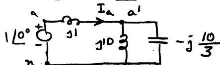
Combining parallel elements we have  $Z_{ll} = -j5$ .  $I_a = 0.25 \angle 90^\circ$
